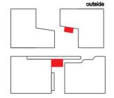
AQUASTRIP cross-sections and sizes are designed to fit all makes and sizes of precast concrete box culverts made to the Box Culvert Association's Standard Specification 1991. Also all precast concrete rebated and ogee pipes BS 5911:110. 5911
