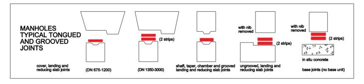
AQUASTRIP cross-sections and sizes are designed to fit the tongued and grooved, rebated or ogee joints of all makes and sizes of precast concrete manhole and inspection chamber sections and slabs to BS 5911 Parts 2 & 200, and BS 5911-1, -3 & -4 and BS EN 1917.
