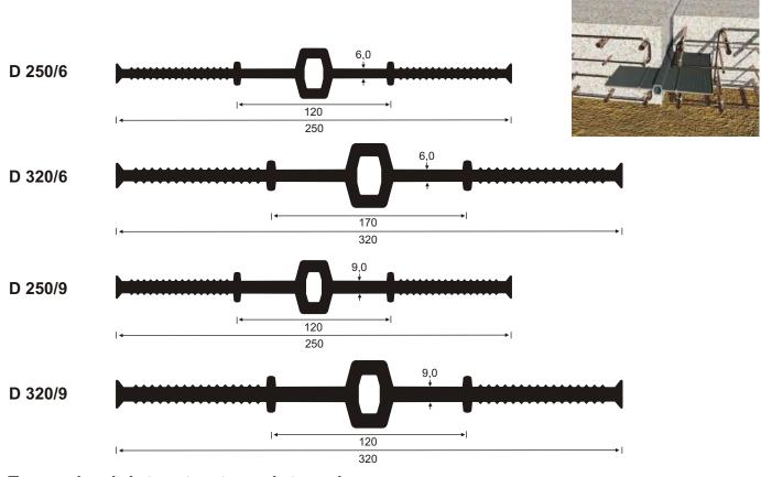
Expansion joint waterstops, internal, with extruded reinforcement and fixing loops, black, LECOTRIL DIN 18541
