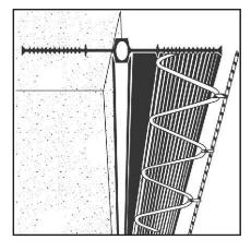
The expansion joint waterstops with fixing loops are reinforced one - sided with harder adjusted PVC - P cords and have fixing loops on both edges of the waterstop.
