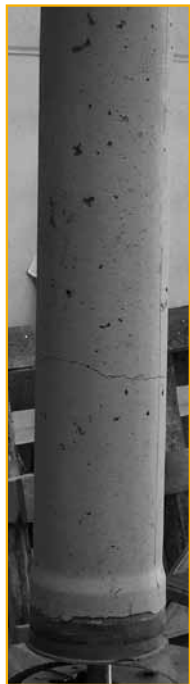
first crack (150 N/mm 2 )
