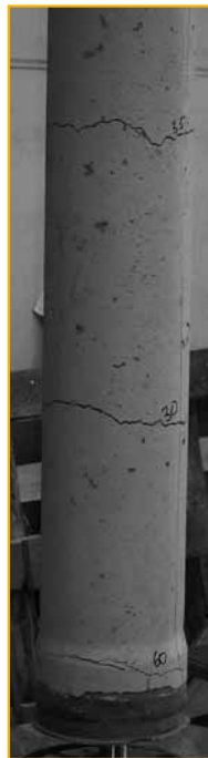
second crack (300 N/mm 2 )
