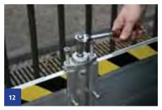
Tighten demountable posts by applying a 10mm socket wrench to the threaded bar located centrally in the top of each demountable post and then swivel the top locking block so that it is positioned over the top of the panels.
